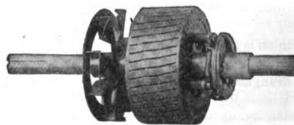
ROTOR SHOWING CENTRIFUGAL OPERATING RING AND VENTILATING PLATE
